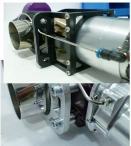
Note the solid fixing of the gearbox to the mounting and through to the firewall, critical in providing a stiff, yet load sharing pathway. This simple but rigid framework provides a lot of engine protection in event of a nose over or crash, however this stress will be passed directly to the firewall so must be a secure point in the airframe.
