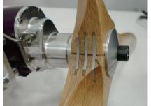
2. Rotate the propeller gently and eyeball the tips from the side to ensure tracking is precise, and correct if not. Any run-out of the tips while under power will generate severe unwanted vibration which can damage the engine.
