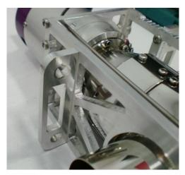
Without such a system any significant prop-strike or nose over could bend the  $2^{nd}$  stage, a very expensive repair.
