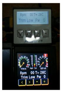
Both displays include dedicated screens for engine operation, radio checking, last shutdown cause and other special turbine operations.
