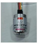
Note: the three wires are <u>NOT</u> the 3phases usually used for a brushless motor. The three wires are for the plus and minus power supply, and a single wire bidirectional digital link.
