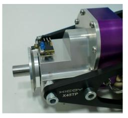
Lubrication for the 2<sup>nd</sup> stage and gearbox is taken from a bleed off the main fuel supply, plus a small air pressure feed to maintain a positive pressure in the gearbox. These are mixed and output via the 2<sup>nd</sup> 4mm swivel fitting on left side of the engine. A small pipe conveys this mixture to an injection point on the gearbox.
