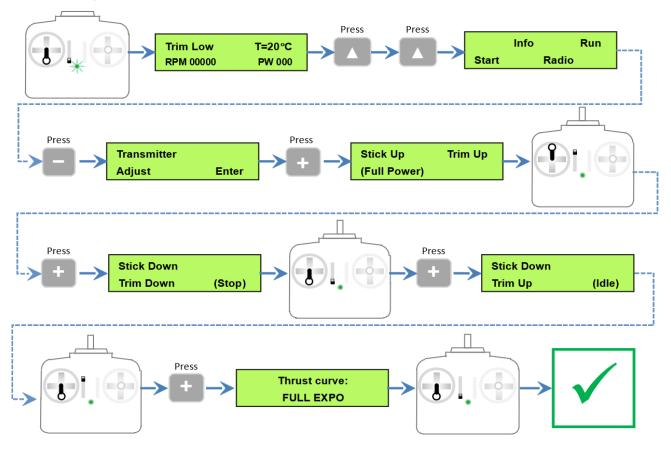
The correct adjustment of the throttle adjustment on the ECU can be verified in the second screen of the display as used before. The percentage of the throttle position should read 0% at the position of engine stop (trim and stick down), 100% with stick/trim full up and between 10% and 30% at idle.
