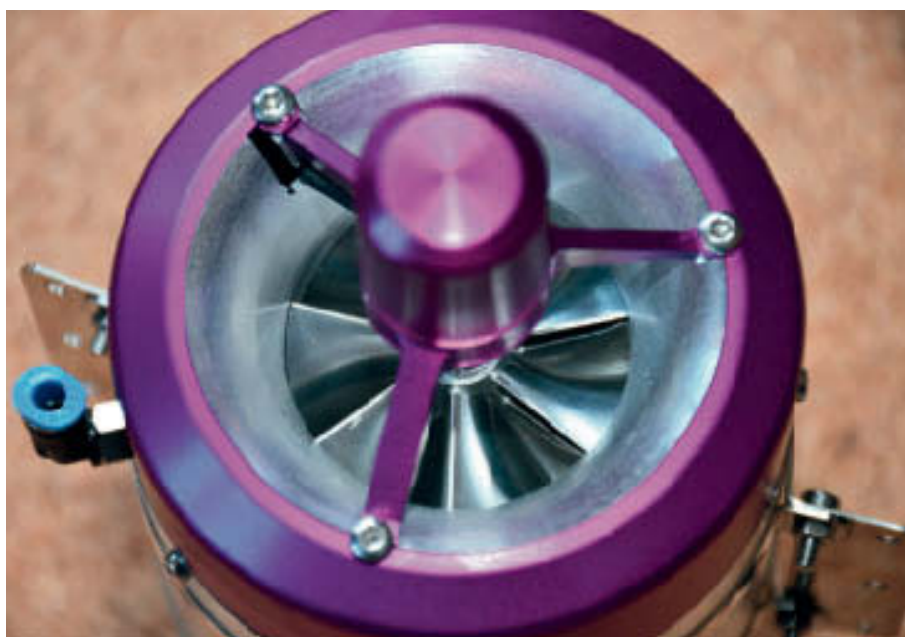
Close up view showing very nice machining on the compressor and the single fuel connector.
