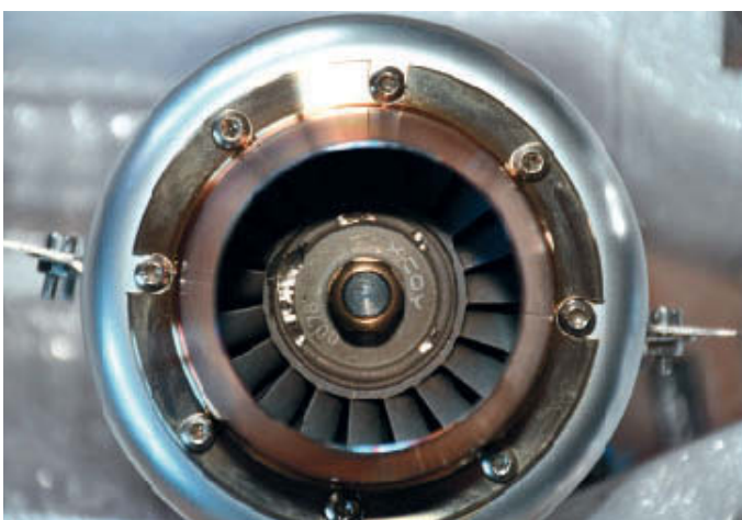
View of the turbine wheel showing the neat casting of the blades and the signs of balancing work.
