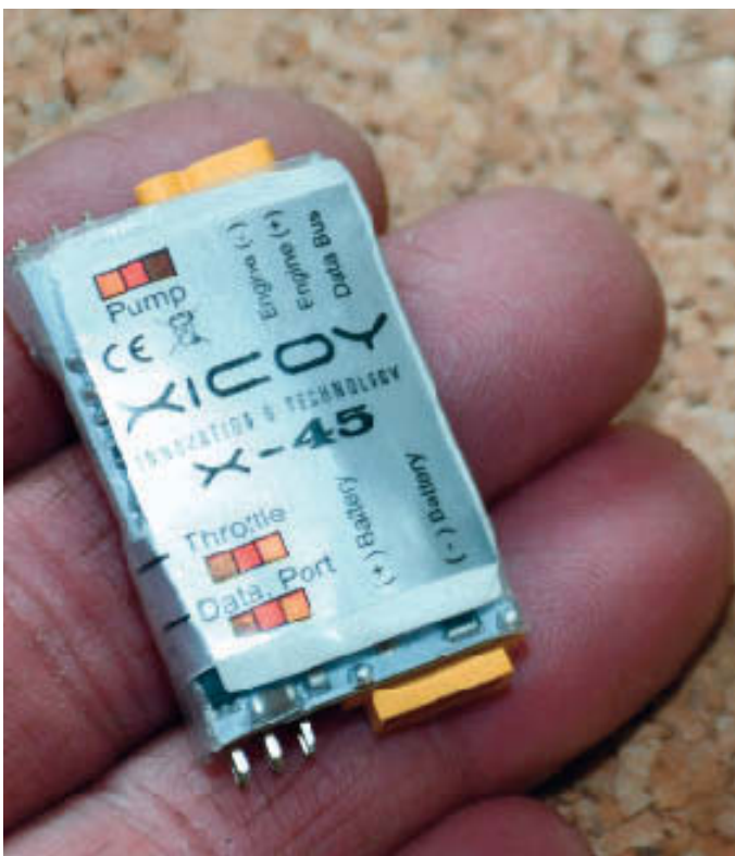
The electronic hub interface connects turbine, battery, fuel pump and telemetry modules/display etc.
