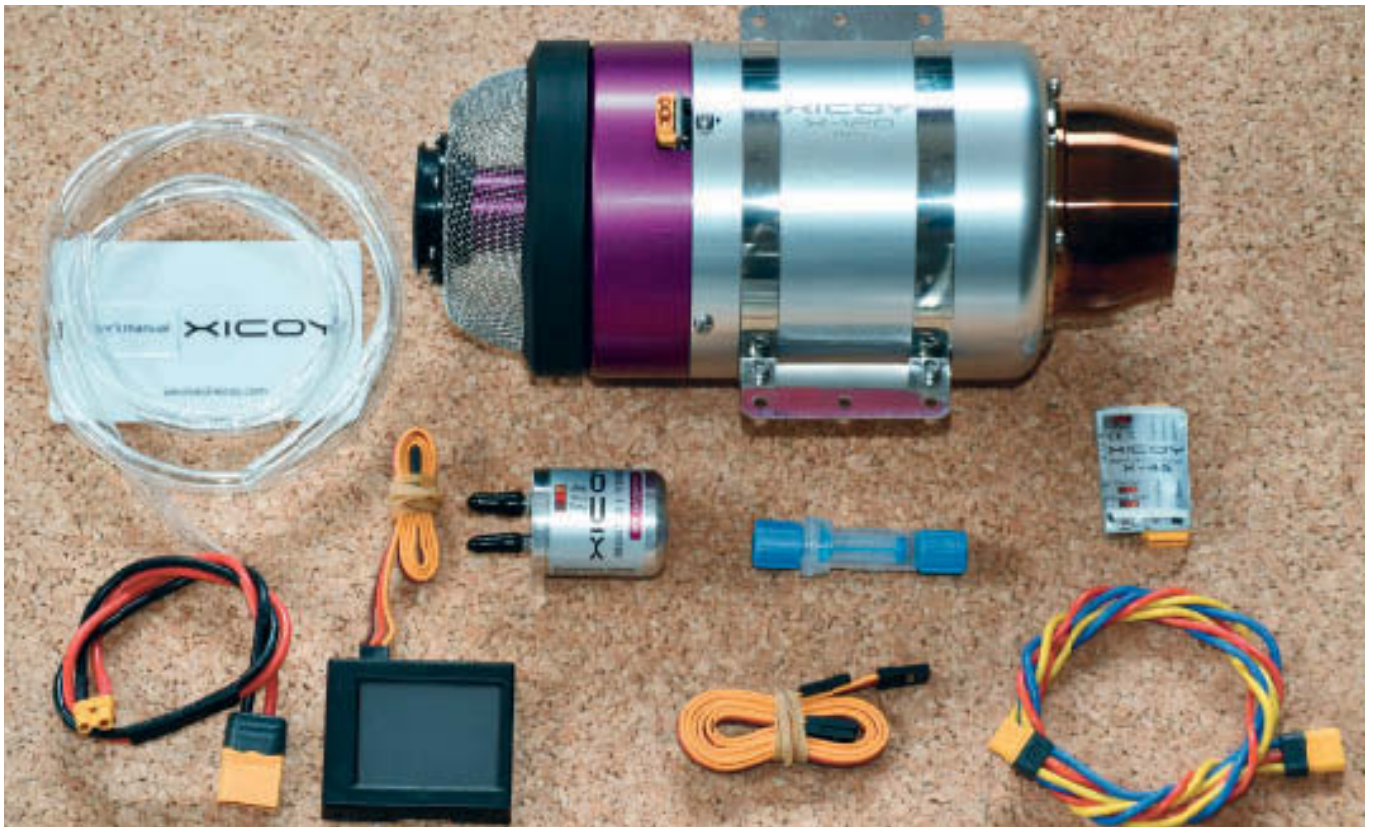
The turbine and main components laid out, note the minimal overall component count given the simplicity of the X120, the digital control system reducing the lead count.
